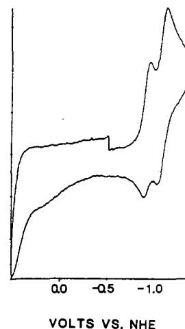
Figure 4. Cyclic voltammetry of 3 mM 2^{2+} in 0.1 M (TBA)PF 6 , CH 3 CN, at v = 20 V/s.
